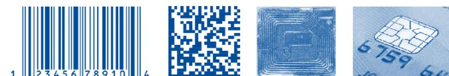
Figure 2. Bar code, 2d bar code, RFID and chip
